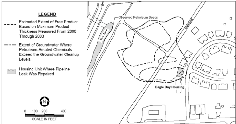
Figure 5 Eagle Bay Housing Area, Estimated Extent of Groundwater Contamination and Residual Free Product
